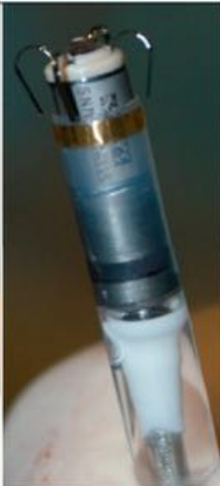
Tines Completely Retroflexed - Micro Still In Sheath
