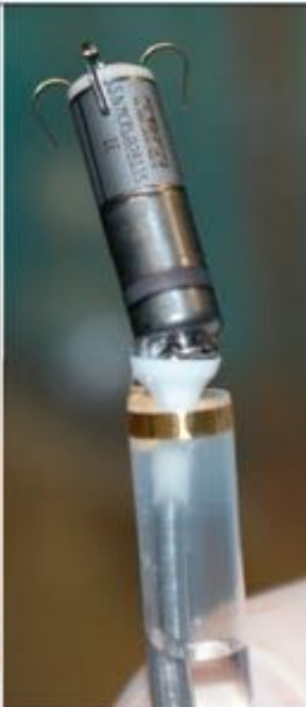
Sleeve Withdrawn - Micro Remains Tethered at Delivery Tool Interface
