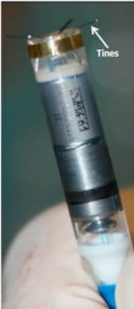
Protective Sleeve Being Withdrawn - Tines Extending
